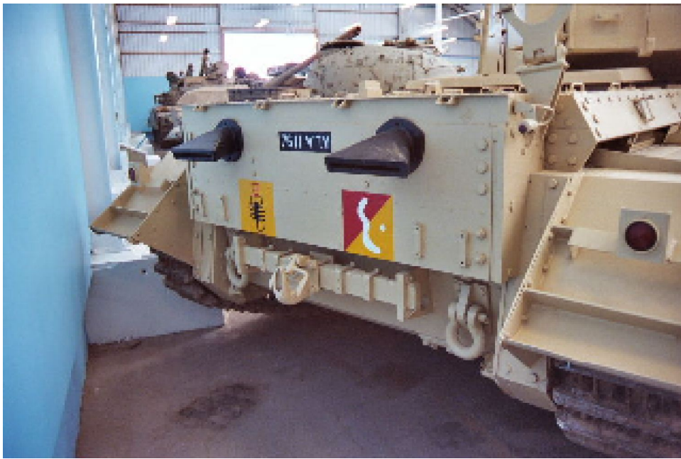
Above, see the exhaust and leaf spring tow mounting position. Below, see the location where the travel lock is welded to the left rear corner of the hull. Note that it ends up being at a slight angle to the hull, so that the travel lock when fitted is aligned with the gun tube.
