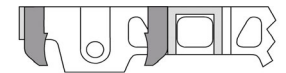
Inside view of bogie frame Note flat back faces of brake shoes face inside
