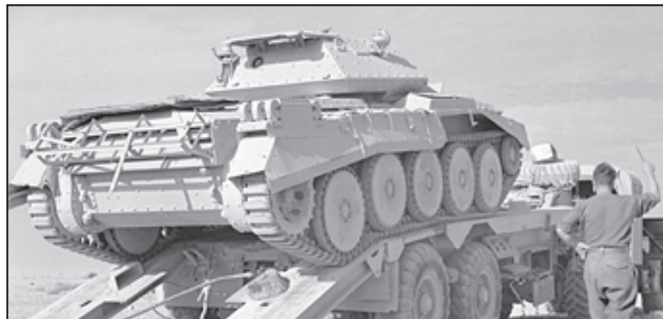
This photo (Imperial War Museum, E-7014) shows the rear turret antenna mount, detail of rear sandshields and on the sloping rear plate, a rack for British 'flimsy' gas cans. Photo via G. Bradford.
